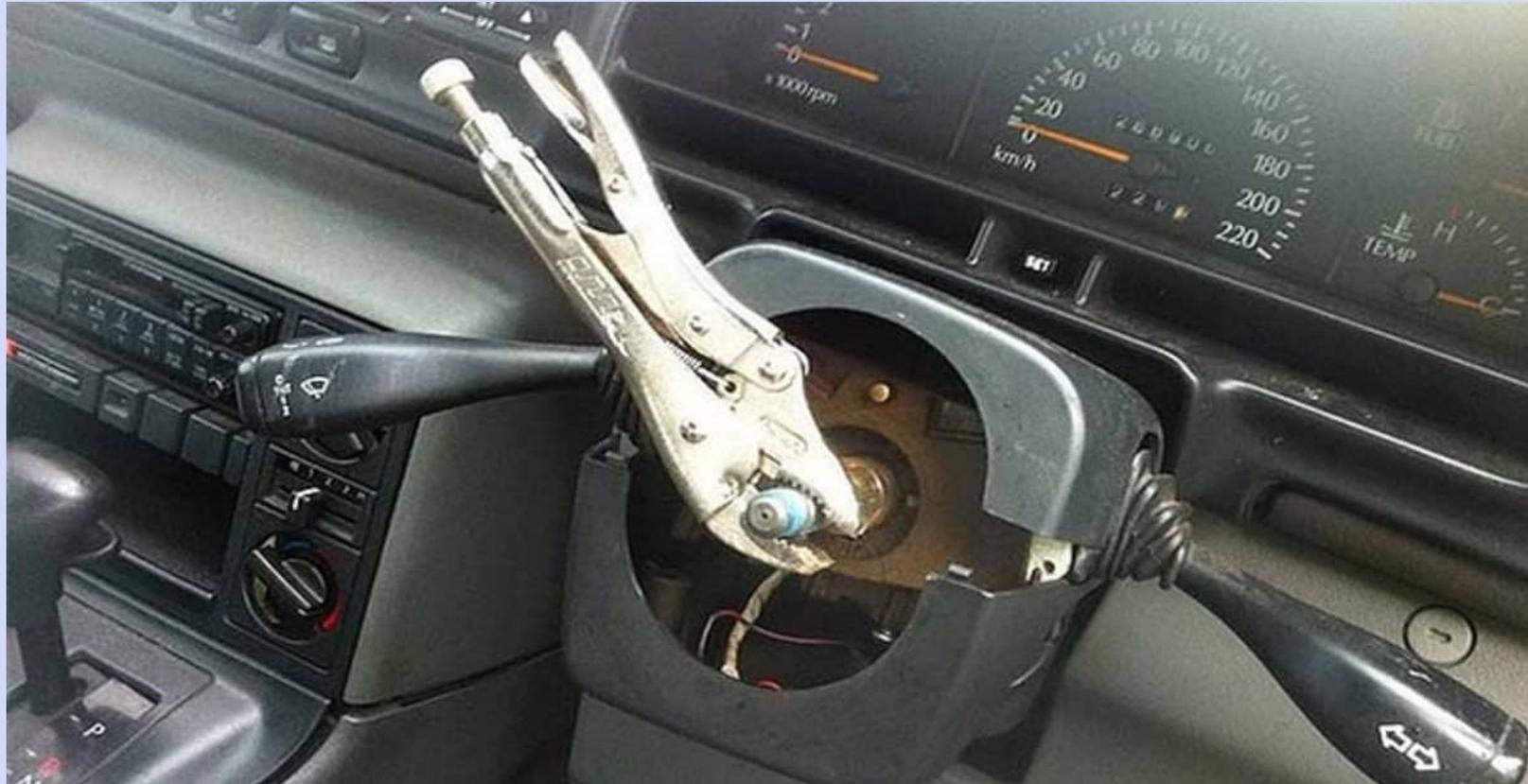
*The inside of a taxi impounded in Rosettenville. The floor has been reconstructed and most of the electronics exposed with additional wires to the ignition, which is activated by a separate button.*
